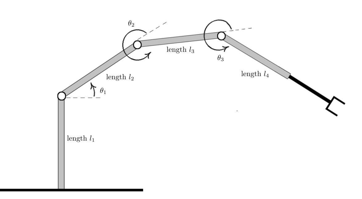
This picture is taken from [1]. Here  $l_1, l_2, l_3$  and  $l_4$  are variables,  $c_1 = \cos(\theta_1), c_2 = \cos(\theta_2)$  and  $c_3 = \cos(\theta_3)$  are parameters and  $s_1 = \sqrt{1 - c_1^2}, s_2 = \sqrt{1 - c_2^2}$  and  $s_3 = \sqrt{1 - c_3^2}$  are the field extensions. The algebraic function field is  $L = \mathbb{Q}(c_1, c_2, c_3)(s_1, s_2, s_3)$ .
