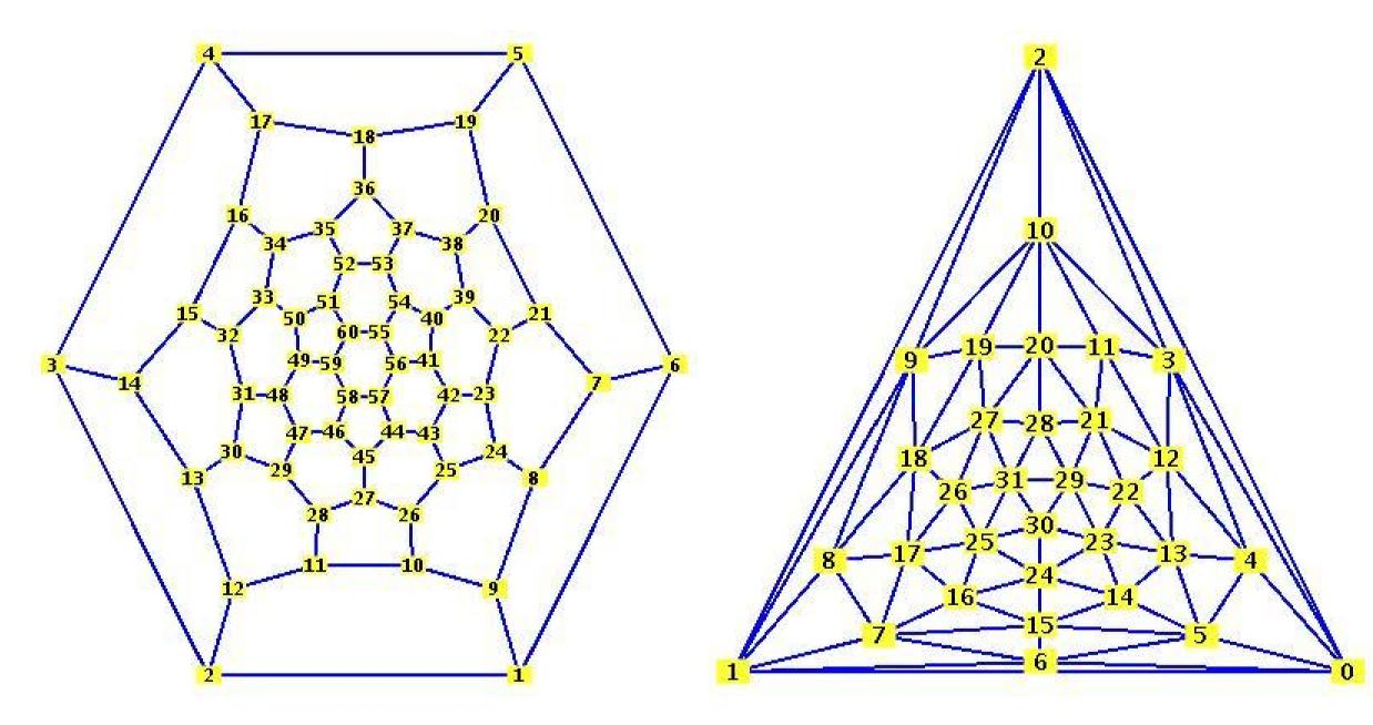
The truncated icosahedron graph G and its planar dual  $G^*$ . Their Tutte polynomials are related by  $T(G, x, y) = T(G^*, y, x)$ .  $T(G^*) = x^{31} + 59 x^{30} + 60 x^{29} y + 1710 x^{29} + \ldots + 160271797870414 y^2 + 11551226205884 y$
