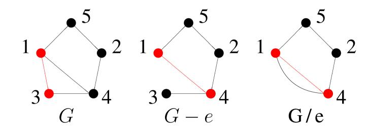
Consider the graph G shown in the figure above. The vertex order heuristic picks the edge e = (u, v) where u is the first vertex in the G and v is the first vertex adjacent to u. In our example u = 1, v = 3, hence e = (1, 3) is chosen. Shown are the graphs G - eand G / e where when we contracted the edge e = (1, 3) we "pulled" vertex 3 down to vertex 1. The next edge selected in G / e will be one of the edges (1,4).
