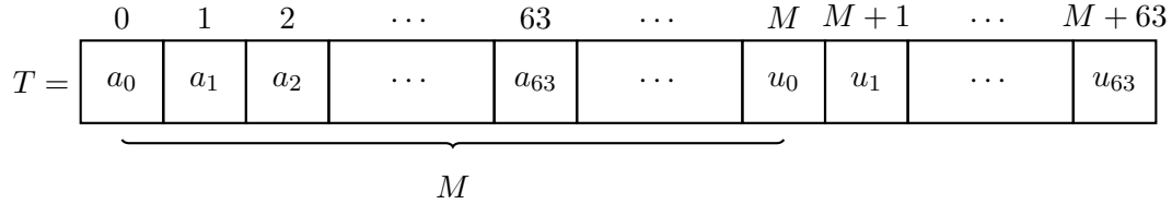
Figure 5.6: The way BUPT stores T_{6,0} - x^{64} in the array T when n = 64
